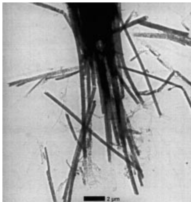
Figure 6. TEM of CNT fibers. The fiberlike, compact nature of the filled tubes is visible from the dark contrast of the single objects.
