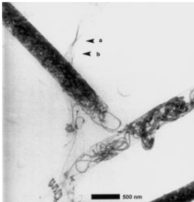
Figure 7. TEM of CNT fibers showing the dense, compact filling of the outer larger CNTs with smaller helicoidal CNTs. The arrows mark a flat and twisted region of an empty, collapsed CNT.
